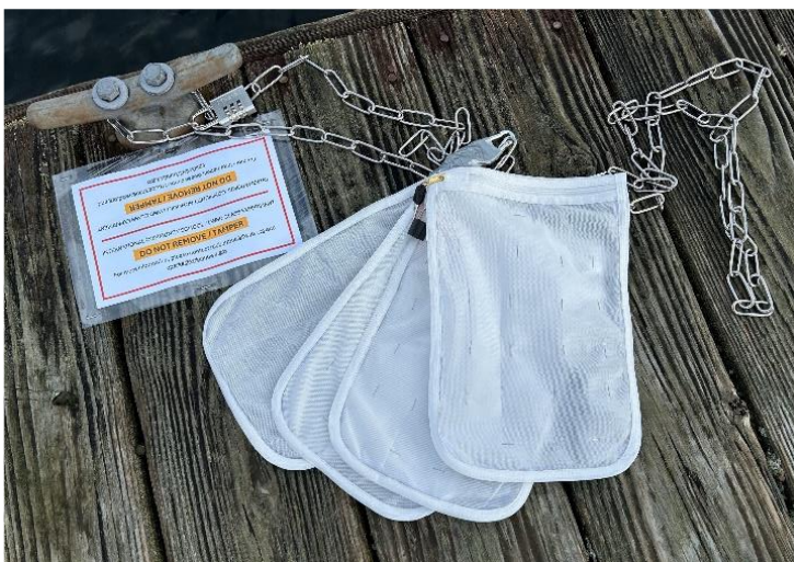
Fig. 3d A Sample Group of Two PET and Two PP Bags Chained to a Dock Cleat
