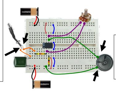
Connect the **output voltage** probes to the two speaker terminals. Be sure the metal tip is in contact with the conducting part of the wire—not the plastic insulation.
